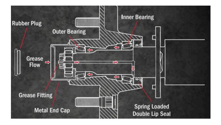
Located at the end of the axle spindle is a grease nipple. This allows you to lubricate the inner and outer bearing by having a pathway from the grease nipple at the end of the axle to the inner bearing. This enables the grease to be pushed towards the outer bearing and into the dust cap.
